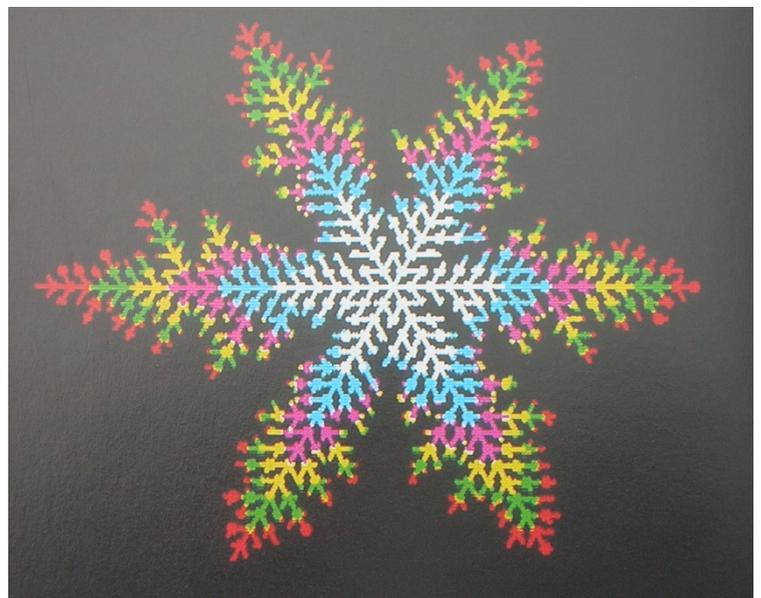
**Determination of the fractal dimension from experiments****Image analysis: Ag grown on Pt(111) at 110 K**
