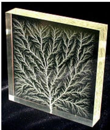
Fig.XXX Lichtenberg figure (from Wikipedia on dendrites). High-voltage dielectric breakdown within a block of plexiglass creates a fractal pattern.
