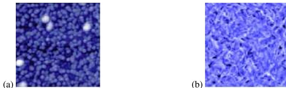
**Figure 3.** Scanning force microscopy images taken in non-contact mode of 1:1 blended films (nominal thickness of 25 nm) of (a) C<sub>60</sub> and CuPc deposited on a SiO<sub>2</sub>/Si substrate (Max. height: 58 nm, RMS roughness: 6.5 nm) (b) CuPc and F<sub>16</sub>CuPc deposited on a PEDOT:PSS coated ITO substrate (Max. height: 15 nm, RMS roughness: 2.0 nm) with a total image size of 2×2 μm<sup>2</sup>.
