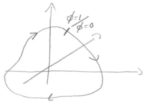
$$\frac{d\phi}{dt} = \omega \frac{V^m}{V^m + V_c^m}$$
