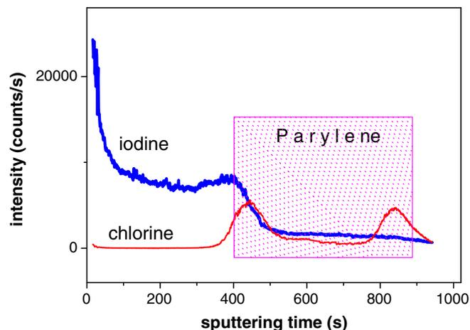
**Fig. 5.** SIMS depth profile of iodine and chlorine in the sample J161 after 48 h of iodine diffusion. The parylene C layer is schematically denoted by a rectangle.
