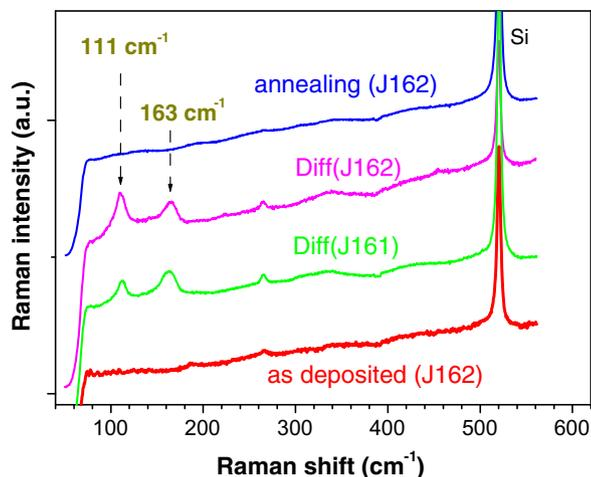
**Fig. 3.** Micro-Raman spectra of iodine doped PEN films J161 and J162 (middle spectra). For comparison the spectrum of J162 is plotted at the bottom for pristine films and on top after iodine diffusion and vacuum annealing. The peaks at  $520\text{ cm}^{-1}$  come from the Si substrate.
