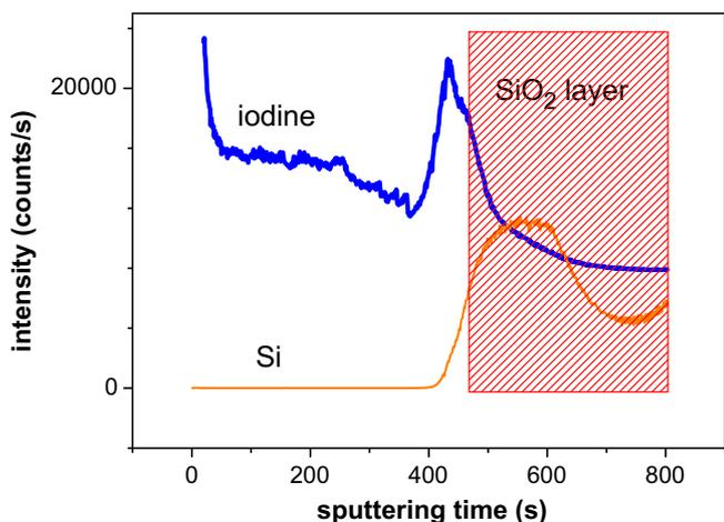
**Fig. 4.** SIMS depth profile of iodine and Si in the sample J162 after 48 h of iodine diffusion. The  $\text{SiO}_2$  layer is schematically denoted by a rectangle.
