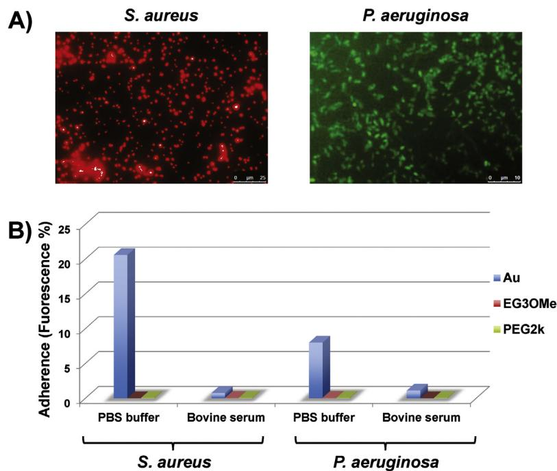
**Fig. 7.** Adherence comparison between *S. aureus* and *P. aeruginosa*. (A) Fluorescence images on uncoated gold (Au) surfaces after incubation with *S. aureus* or *P. aeruginosa* in PBS buffer. (B) Comparison of the cell counts on uncoated gold (Au) surfaces, EG<sub>3</sub>OMe coated and PEG2k coated surfaces for *S. aureus* and *P. aeruginosa* resuspended in PBS buffer or bovine serum.
