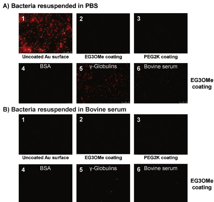
**Fig. 4.** Effect of *S. aureus* resuspended in PBS buffer (A) or serum (B) on adherence to EG<sub>3</sub>OMe and PEG2k coated surfaces. Fluorescence microscopy images of *S. aureus* (pC-tuf-ppmch) adhered on uncoated Au surface (1), EG<sub>3</sub>OMe coating (2), PEG2k coating (3) and EG<sub>3</sub>OMe coating pre-incubated with 20 mg/ml BSA (4), 50 mg/ml  $\gamma$ -globulins (5) or 100% bovine serum (6).
