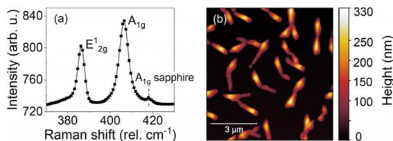
**FIG. 1.** (a) Raman spectra of the MoS<sub>2</sub> monolayer on the sapphire substrate. Two characteristic Raman vibrational modes of MoS<sub>2</sub>–E<sub>2g</sub><sup>1</sup> and A<sub>1g</sub> are labeled. The peak at  $\sim 417.9 \text{ cm}^{-1}$  is attributed to A<sub>1g</sub> of the sapphire substrate. (b) AFM image of the DIP crystals on the MoS<sub>2</sub> monolayer.
