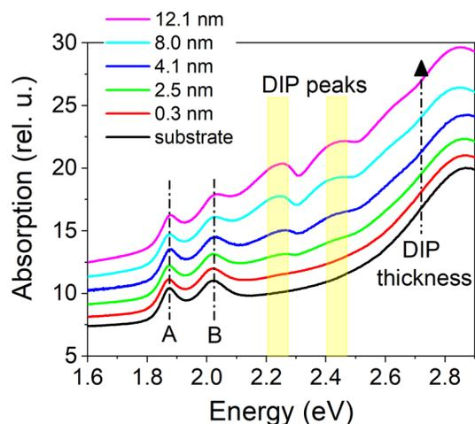
**FIG. 4.** Absorption spectra of DIP layers with different thicknesses grown on the MoS<sub>2</sub> monolayer. A and B denote the excitonic transition bands for the MoS<sub>2</sub> monolayer at 1.88 eV and 2.02 eV, respectively.<sup>49</sup> Absorption spectra are vertically shifted for clarity.
