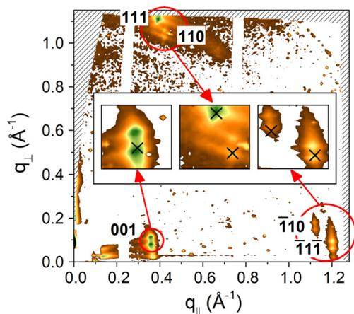
**FIG. 2.** The  $q$ -space map of the 12 nm thick DIP layer on the MoS<sub>2</sub> monolayer (intensity increasing from brown to green). The 001,  $\bar{1}10$ ,  $\bar{1}\bar{1}\bar{1}$ , 110, and 111 diffraction peaks are magnified for a better resolution. The black crosses indicate the calculated positions of the diffraction peaks, using the determined unit cell parameters.
