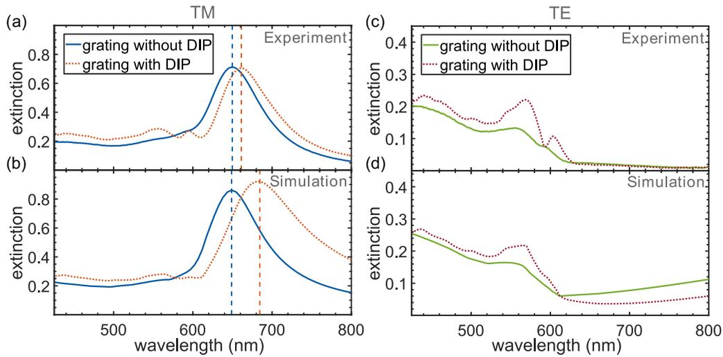
FIG. 2. Experimental [(a) and (c)] and simulated [(b) and (d)] extinction data of gold nanogratings for TM [(a) and (b)] and TE polarization [(c) and (d)]. The solid blue and green curves show the spectra without DIP, and the dotted orange and red curves the spectra of the hybrid system. The vertical dashed lines indicate the positions of the LSPRs.
