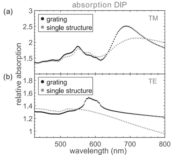
FIG. 4. Simulated relative absorption of the DIP layer on a grating and a single wire, respectively, relative to DIP directly on a glass/ITO substrate for (a) TM and (b) TE polarization. Values larger than 1.0 correspond to absorption enhancement in the organic layer.
