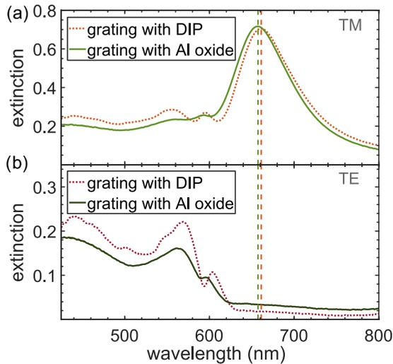
FIG. 3. Comparison of the extinction of gratings covered with DIP (dotted orange and red curves), as in Figs. 2(a) and 2(c) and with aluminum oxide (solid bright and dark green curves) for (a) TM and (b) TE polarization. The vertical dashed lines indicate that the LSPRs for the two hybrid systems in (a) are nearly identical.
