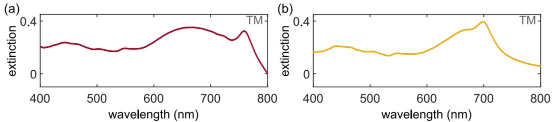
FIG. 6. Experimental extinction spectra of gold gratings with about (a) 500 nm and (b) 700 nm period and a 20 nm DIP film, measured with TM polarized illumination under perpendicular incidence. The parallel lattice modes (a) on the substrate side and (b) on the DIP/air side are clearly visible at about 750 and 700 nm.
