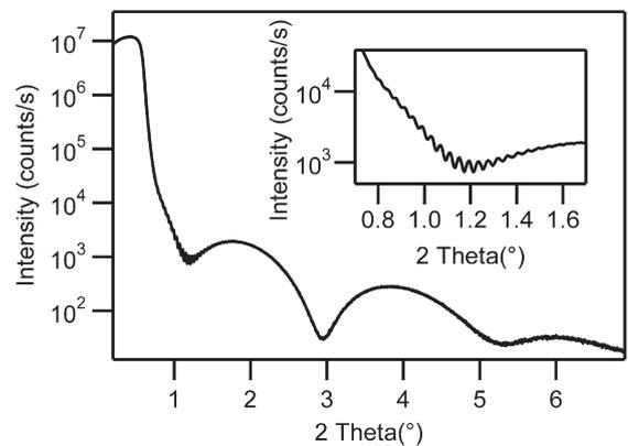
**Fig. 4.** X-ray reflectivity of the Si–Ti–SiO<sub>x</sub> substrate, measured using Cu Kα radiation. The interference fringes demonstrate the formation of well-defined interfaces and reveal the thicknesses of the SiO<sub>x</sub> and Ti layers. The narrow fringes (enlarged in the inset) correspond to a Ti thickness of 212 nm, whereas the broad fringes yield an SiO<sub>x</sub> thickness of 6.4 nm.
