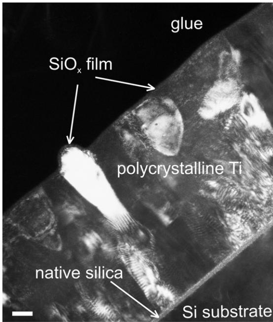
Fig. 1. Dark field TEM image of cross-sectional Si-Ti-SiO<sub>x</sub> specimen. Scale bar represents 20 nm.
