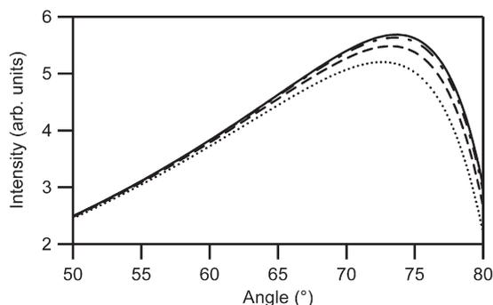
Fig. 5. Simulation of the PM-IRRAS signal from an organic thin film (15 nm thick) which is separated from a semi-infinite titanium substrate by a silicon oxide film of thickness: no silicon oxide (—), 5 nm (– · – ·), 20 nm (– – –), 50 nm (·····).
