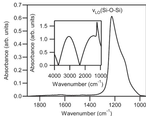
Fig. 6. PM-IRRAS spectrum of non-functionalized Si–Ti–SiO<sub>x</sub> substrate. Inset shows spectrum before, and main figure after removal of the Bessel function envelope.
