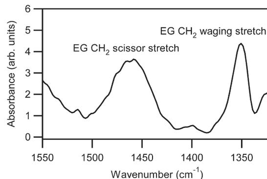
Fig. 7. Background-subtracted PM-IRRAS spectrum of Si–Ti–SiO<sub>x</sub> that has been functionalized with silane–PEG–biotin.
