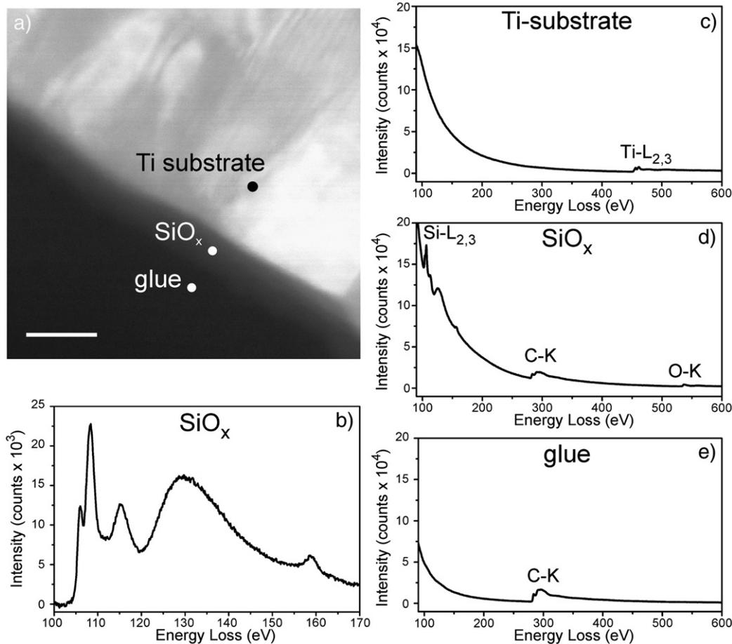
Fig. 2. HAADF-STEM and EELS characterization of Si-Ti-SiO<sub>x</sub> substrate. a) HAADF-STEM image of a cross-sectional TEM specimen. Scale bar represents 20 nm. c) d) e) EELS spectra recorded in the energy range of Si-L<sub>2,3</sub>, C-K, Ti-L<sub>2,3</sub> and O-K edges from the regions indicated in image (a). b) Background-subtracted Si-L<sub>2,3</sub> edge acquired at a position similar to that of (d).
