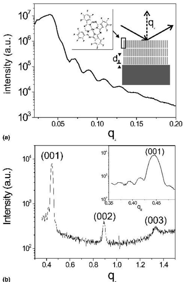
Fig. 1. (a) X-ray reflectivity data of a F<sub>16</sub>CuPc thin film. The inset shows a scheme of the molecule and of the specular diffraction geometry. (b) X-ray diffraction along the specular rod showing the three first order Bragg reflections. Inset is the rocking scan in the (001) Bragg peak; Laue oscillations appear at the sides of the peak.
