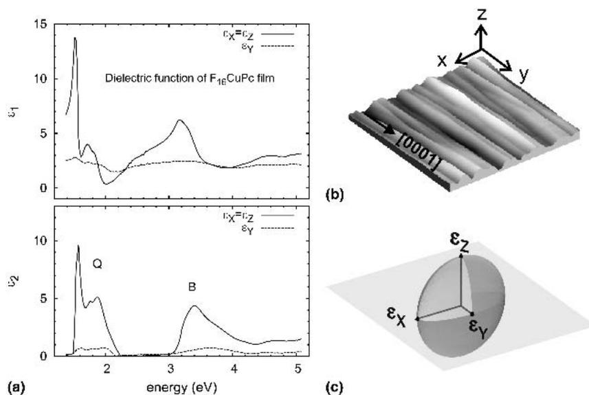
FIG. 4 (a) Fitted in-plane dielectric functions for one of the films denoted  $\epsilon_x$  (component along substrate's  $[1\bar{1}00]$  direction, perpendicular to the wires) and  $\epsilon_y$  along  $[0001]$ , in this case along the wires). (b) AFM topographical image of this film. (c) Scheme showing the indicatrix or real part of the dielectric tensor obtained for this sample at 3 eV.
